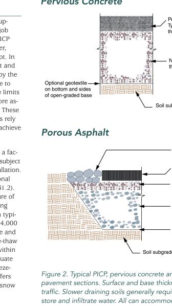
Typ. No. 8 aggregate in openings PICP Curb/edge restraint with cut-outs for overflow drainage Concrete pavers min. 3 <sup>1</sup>/<sub>8</sub> in. (80 mm) thick Bedding course 11/2 to 2 in. (40 to 50 mm) thick 4 in. (100 mm) (typ. No. 8 aggregate) thick No. 57 stone open-graded base No. 2 stone subbase - thickness varies with design Optional geotextile on bottom and sides of open-graded base Soil subgrade **Pervious Concrete**
