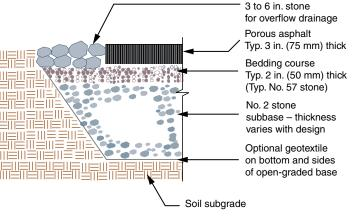
Figure 2. Typical PICP, pervious concrete and porous asphalt pavement sections. Surface and base thicknesses vary with traffic. Slower draining soils generally require thicker bases to store and infiltrate water. All can accommodate perforated drain pipes in the base for low infiltration soils.
